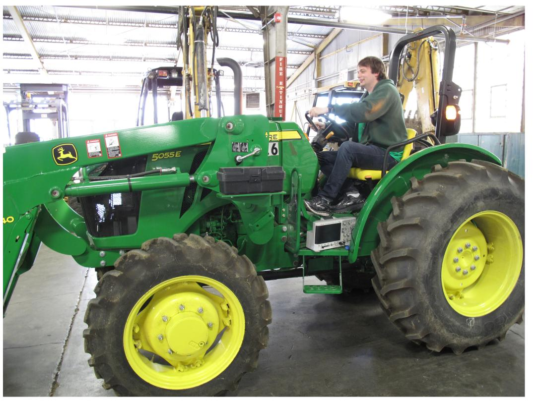
The tractor used for live tests is a John Deere 5055E model, which is a fairly simple open-cab tractor. As a result, the computer architecture inside it is not incredibly complex. The tractor has a CAN port to which we connected our MSO-X 2012A Keysight oscilloscope. This scope is able to identify a message sent in the CAN format, break it up into its ID and data components, and save ten seconds of this data to a flashdrive.
